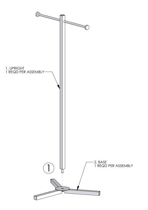
${\rm D}$  screw the upright into the threaded hole in the center of the base. Use the faceouts of the upright to help tighten.
