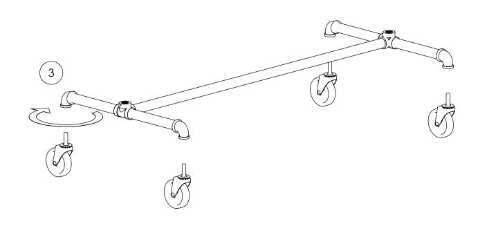
SCREW IN THE CASTERS TO THE BASE AS SHOWN USING PROVIDED WRENCH
