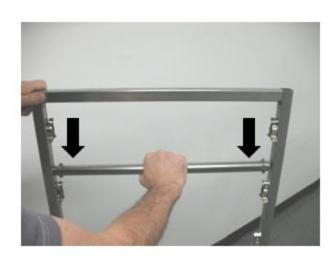
**3.** Clip each of the six hanger bars onto the rack clips as shown.
