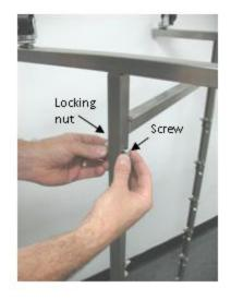
2. Secure the legs to the frame using the supplied screws and locking nuts. Fully tighten using a phillips head screwdriver and a 7/16" or adjustable wrench.
