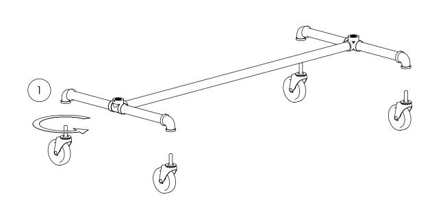
SCREW THE CASTERS INTO THE BASE AS SHOWN USING PROVIDED WRENCH
